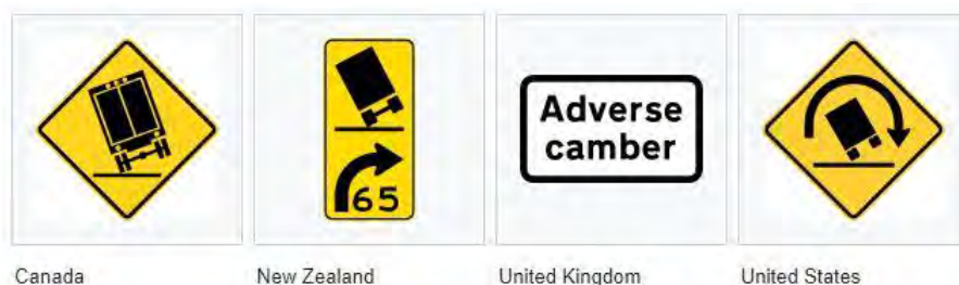
Figure 1. Signs for warning curves with an increased danger of rollover (Google Image).
