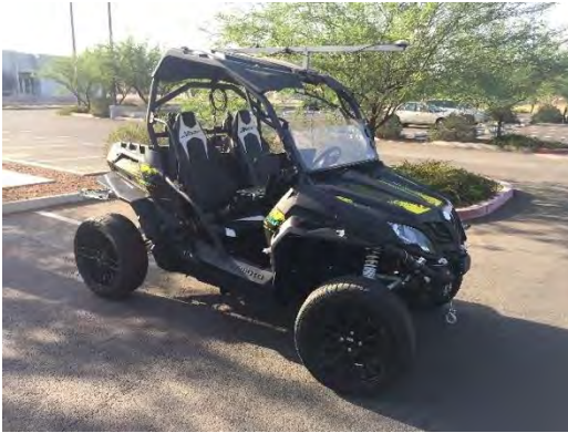
Figure 31. 4IWM AGV prototype and vehicle parameters.
